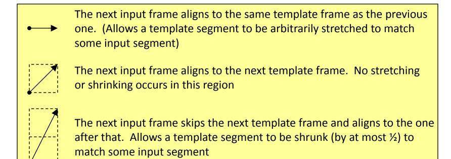
• Note that all transitions move one step to the right, ensuring that each input frame gets used exactly once along any path
